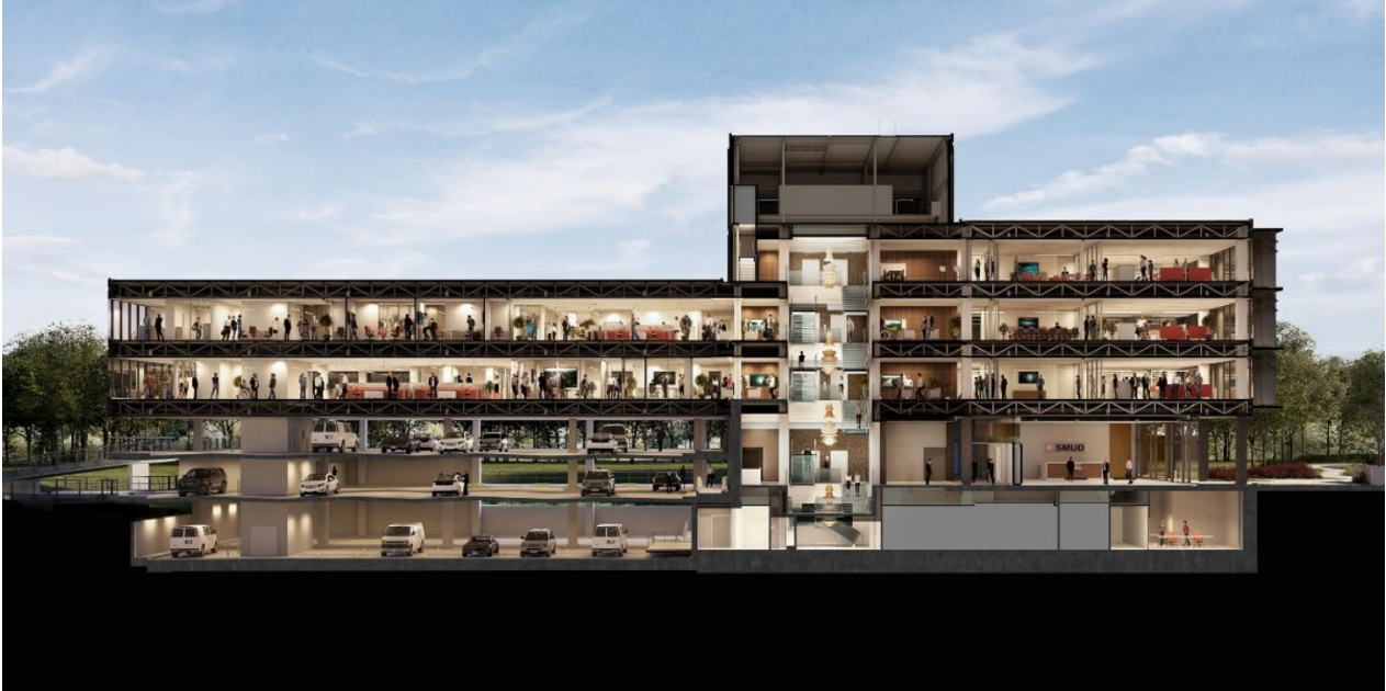
Renderings and historic photography courtesy of Dreyfuss + Blackford Architecture. Caption: Section of building showing lower level parking, open offices, central stair and reception.
